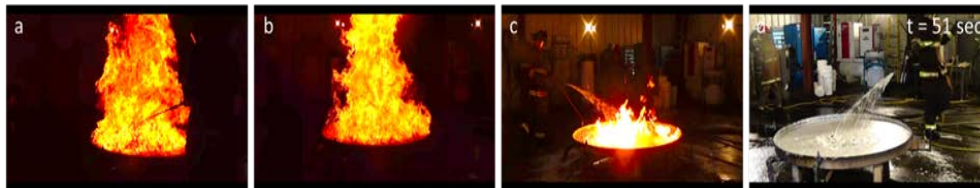
Testing Fluorine Free Foams: Performance improving, still lag behind AFFF
